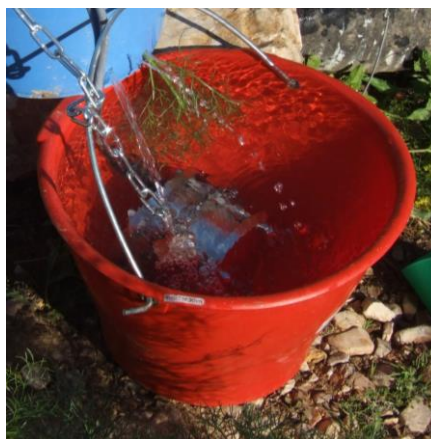
Figure 5: Field fluorimeter in a through-flow cell (bucket)
