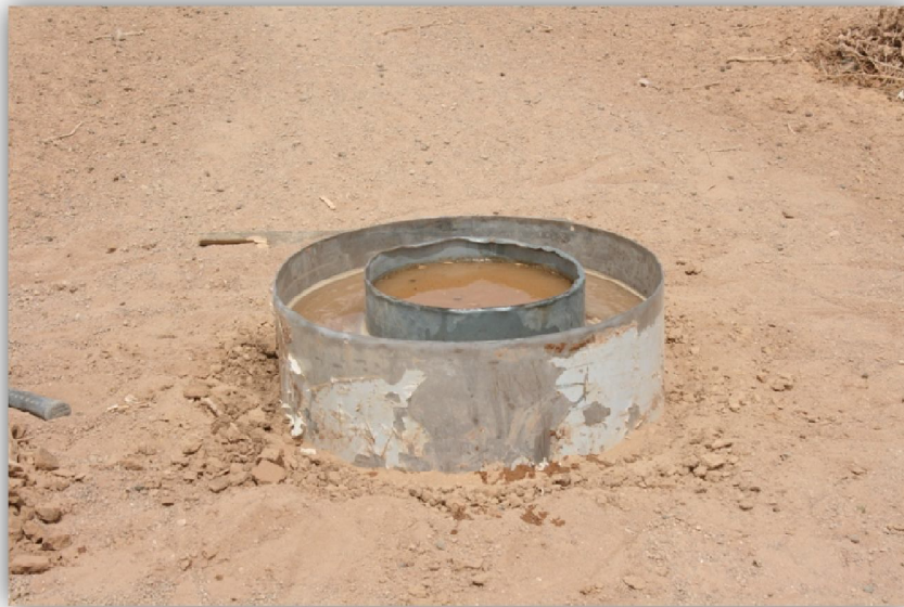
Photo: 38: Implementation of second DRIT in Wadi Dhuleil site.
