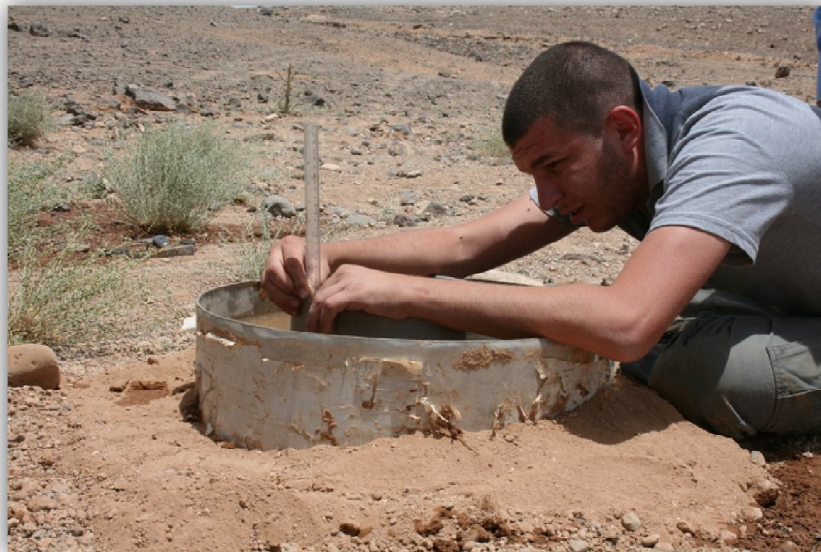
Photos 28: Implementation of second DRIT in Mafraq safawi Eastern site.
