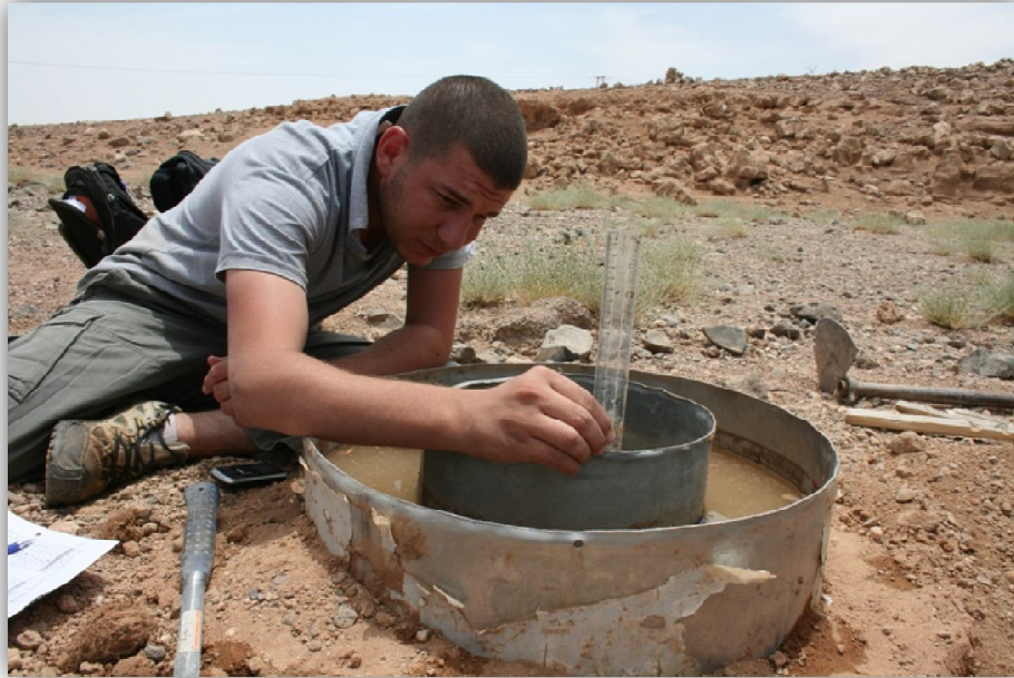
Photos 26: Implementation of first DRIT in Mafraq safawi Eastern site.
