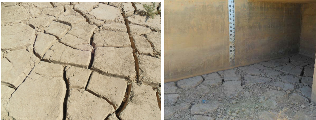
Fig. 44: Sediment accumulation with mud cracks at Wadi Madoneh dam (M2) of about 40 cm at dam wall. (Pictures taken by A. Steinel, 2011).
